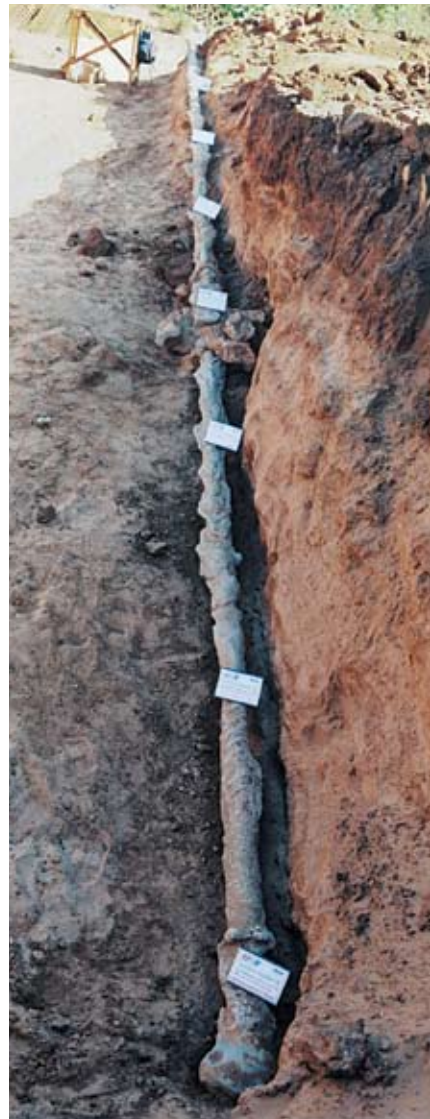
Grouting body built by using the AT - RIA Rotary-Injection-Adapter
